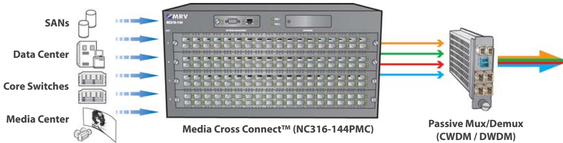
Figure 3: NC316-144PMC as high-density, multi-rate transponder for WDM applications
