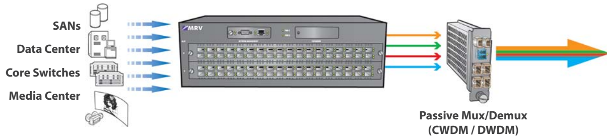
Figure 3: NC316-72PMC as high-density, multi-rate transponder for WDM applications
